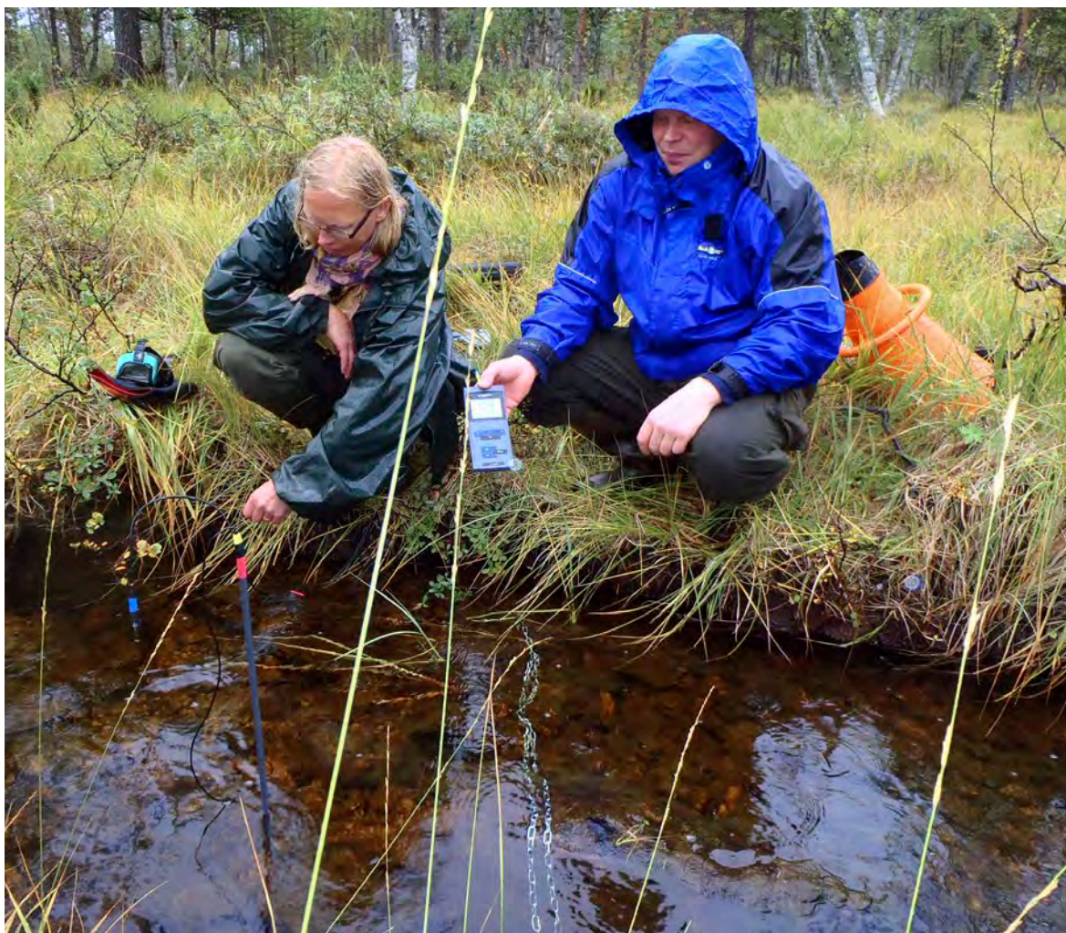
Figure 2a. Measuring redox potential ( E_h ) from the interstitial water with a redox probe (red marking) and reference probe (blue marking). The redox probe was pushed 5 cm or 10 cm deep down in the sediment (see Fig. 2b). Photo Panu Oulasvirta, Metsähallitus.
