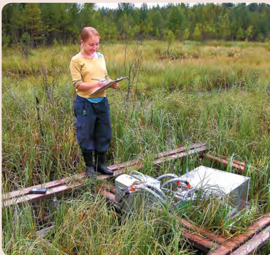
**Figure 8.** Measuring carbon dioxide flows in a restored fen. The amounts of carbon absorbed and released can be measured using closed chambers. PHOTO: JUKKA LAINE.
