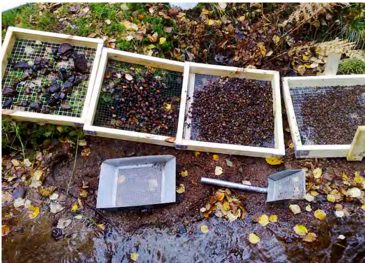
Figure 20. Series of sieves (mesh size 19 mm, 12 mm, 5 mm and 2.5 mm from left to right) and sediment excavation tools used in juvenile pearl mussel search in the River Ijoki area in September 2013.
