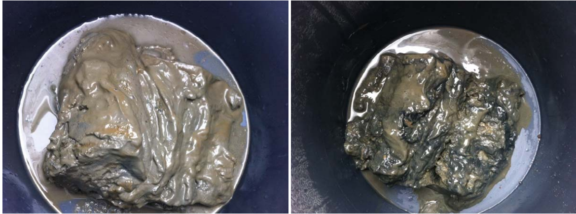
Figure 3. Samples were visually described based on colour and smell. The picture to the left shows a healthy and “normal” sample, whereas the sample to the right is considered affected showing signs of oxygen deficiency. Photos: Anna Arnkil/Metsähallitus.
