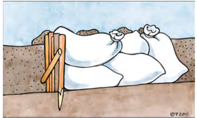
Figure 38. Jute sacks filled with compressed peat can be put in place manually to dam ditches with sensitive springs or seepage areas, for instance. Such sack dams are also suitable for use when repairing dams in restored sites where excavators can no longer work. Sacks can be fixed in place using wooden stakes hammered into the peat.
