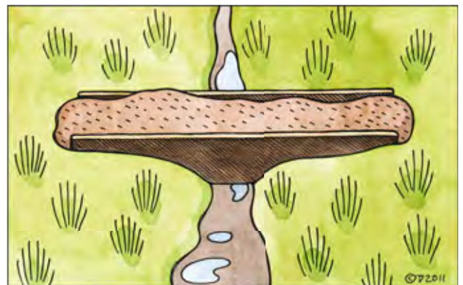
Figure 39. Dams made of plywood can be used to block shallower ditches. Board should be sawn to sizes with greater length and depth than the ditch. To put them in place grooves can be cut in the peat using a long-reach motor-saw. The boards can then be hammered into place e.g. with a sledgehammer. Peat should then be shoveled in between the boards and packed tightly. ILLUSTRATIONS: TUPU VUORINEN.
