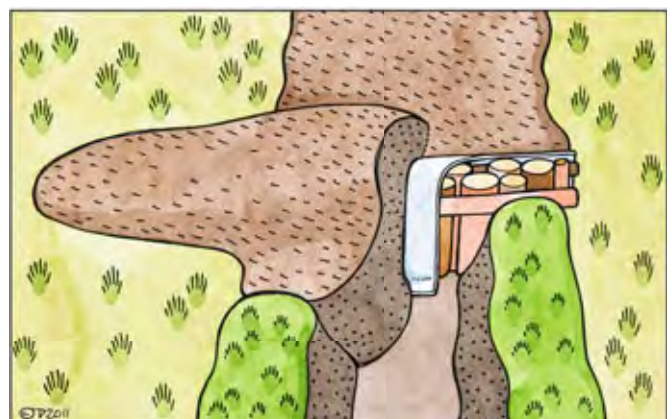
Figure 36. Log dams may be constructed where suitable logs can be cut from trees felled on the site. The top ends of the logs should stand out clearly above the level of the ditch banks. If the peat is deep, the logs can be sunk vertically into the peat, but where peat deposits are only shallow the logs can be put in place horizontally. The dam should then be covered with geotextile and peat. Log dams can be further stabilised with the help of supporting logs aligned at right angles to the other logs. ILLUSTRATIONS: TUPU VUORINEN.
