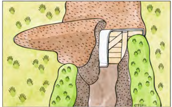
Figure 35. Tongue-and-groove boards can be used to help make dams in large or badly eroded ditches. The geotextile used to cover the boards is only partly shown in these illustrations to enable their underlying structures to be seen. Illustrations: Tupu Vuorinen.
