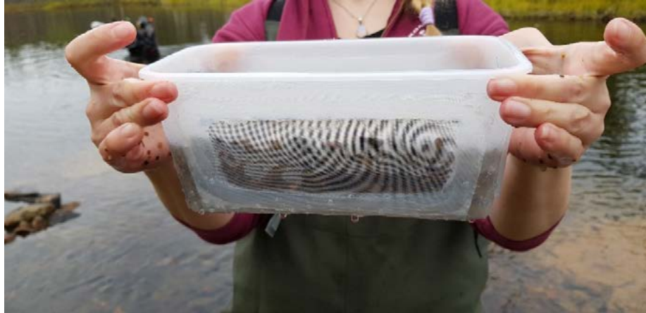
Figure 221. Transplantation box filled with gravel collected and sieved from the bottom of Lutto River. Photo: Jouni Taskinen.
