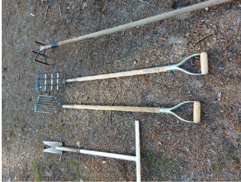
Figure 19. Tools used in Hartijoki method. A "claw" for softening of hardened stream bed below, sieving tools for different-sized gravel in the middle, and a "hoe" for moving stones on the top. Photo: Pirkko-Liisa Luhta.
