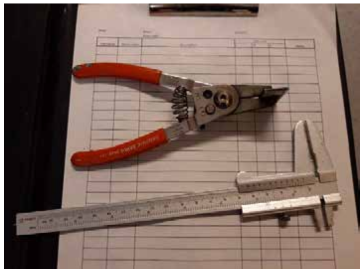
Figure 224. Shell opening tongs specifically constructed to aid opening of the valves of Margaritifera margaritifera shell.
