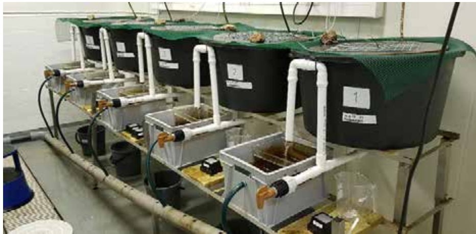
Figure 216. Juvenile collection tanks, enabling emptying from bottom and sieving of out-flowing water for freshwater pearl mussel glochidia. Photo: Jouni Taskinen.
