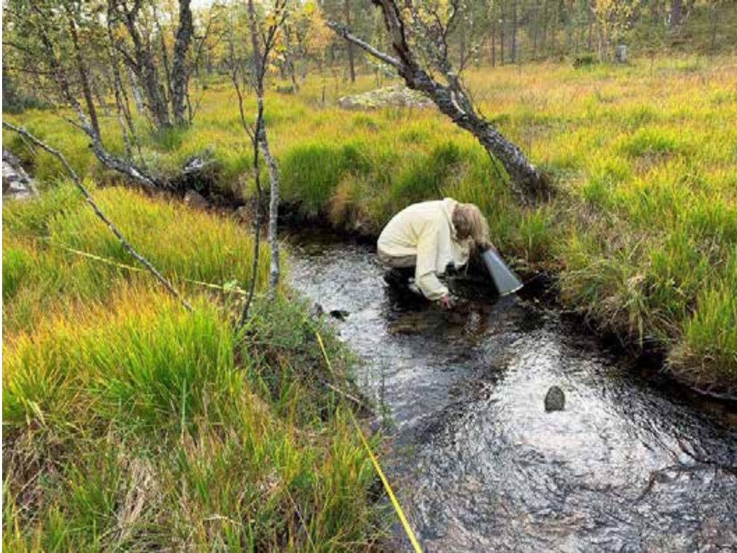
Figure 27. Aquascope was used in the shallowest transects. Here in the river Urakajärvenoja on 31.8.2019. Measuring tape on the riverbank marks the 20 metres long line. Photo: Panu Oulasvirta.
