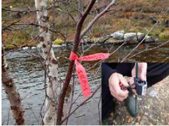
Figure 244a. The loggers were attached into the riverbed with a metal rod. Logger locations were marked. In the picture logger attaching system used by MH. b. Jonna Kuha (JyU) offloading data from a logger in the field in August 2021. Photos: Aune Veersalu.
