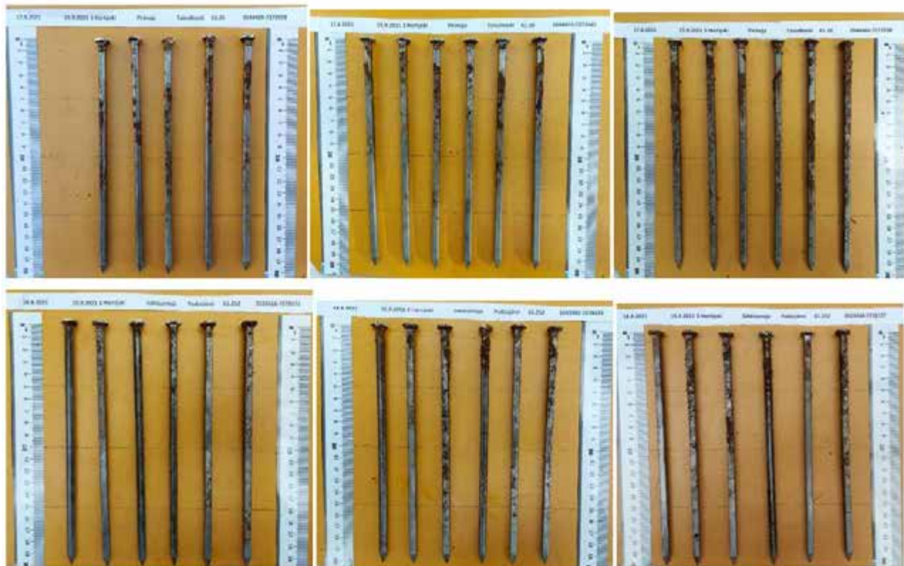
Figure 22. An example of nail test results of Pirinoja and Säkkinenoja based on photographs. Photos: Pirkko-Liisa Luhta.
