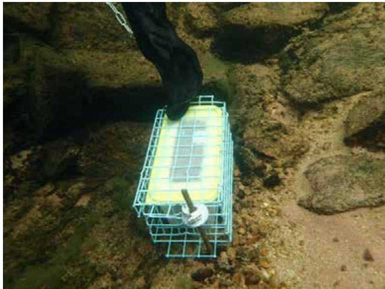
Figure 222. Transplantation box (gravel box) installed on the bottom of Lutto River. Photo: Aune Veersalu.
