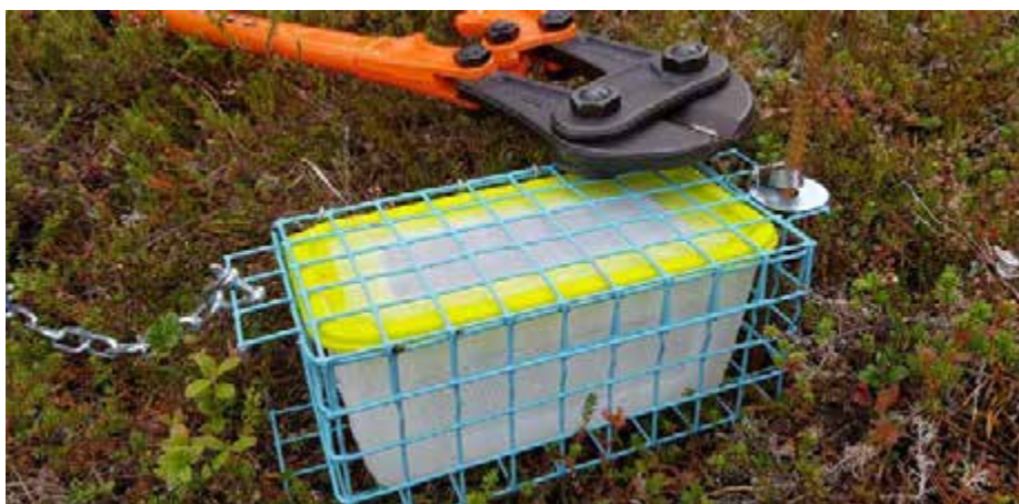
Figure 220. One-liter plastic box with large holes in the sides and lid covered with 200 \mu m plastic mesh to provide flow of fresh river water into the box. The box is kept in a metal protection net to protect the box against physical damage. Metal pole with associated fixing elements, which anchors the box to the bottom is on the right side of the box. Photo: Jouni Taskinen.
