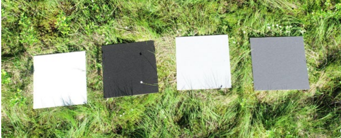
Figure 16. Radiometric calibration panel set. In the project, four MosaicMill 50 cm × 50 cm panels (reflectivity 2%, 9%, 23% and 46%) were mainly used to calibrate multispectral scans. The reflectivity of the panels should be in the same range as that of the site being surveyed. A single panel is usually sufficient for calibration, but with several panels, the calibration can be verified. When capturing images, the lighting of the panels should be similar to the lighting on site. In this image, plants and their shadows partly cover the panels, but even in this case, most of the panel surface area can be used for calibration. Photo: Maarit Similä.
