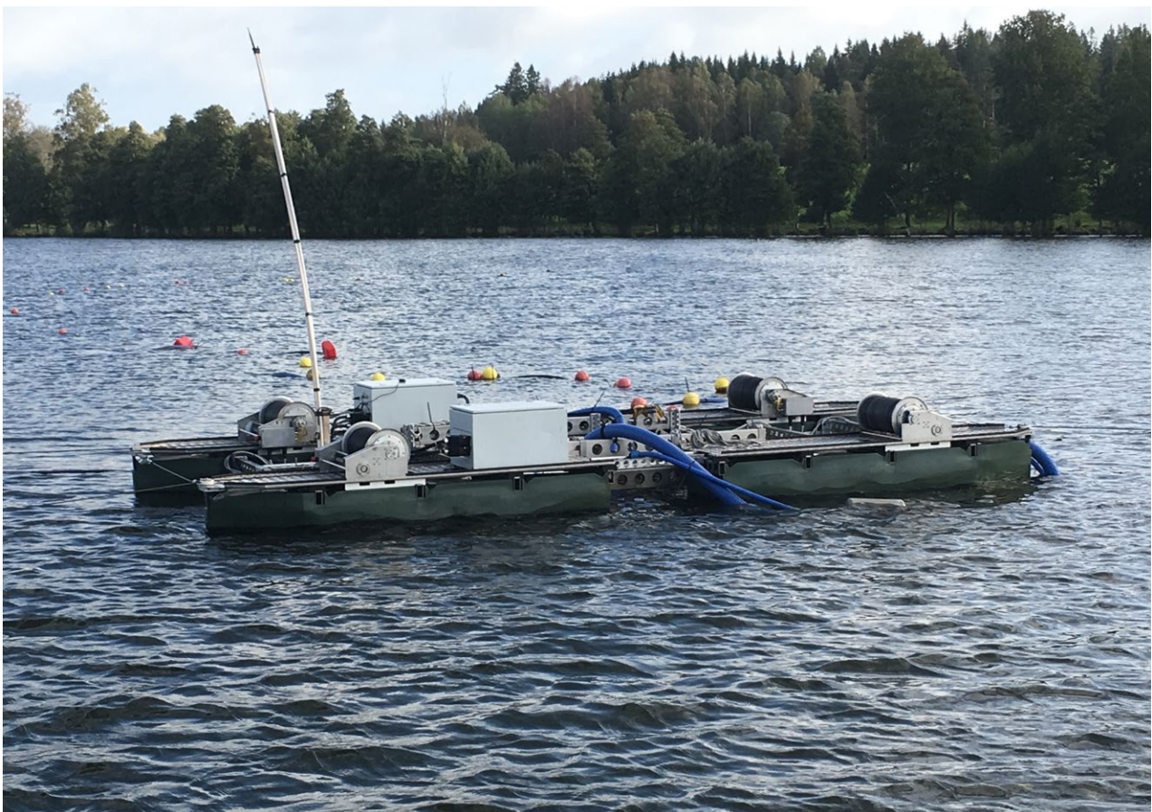
Figure 50. Sediment removal in Jönköping, Sweden (Barnarpasjön) 2018 with low-flow suction dredging equipment. Photo: Irma Puttonen/Åbo Akademi.
